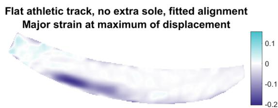
Figure 32: *Strains in standard sole*
